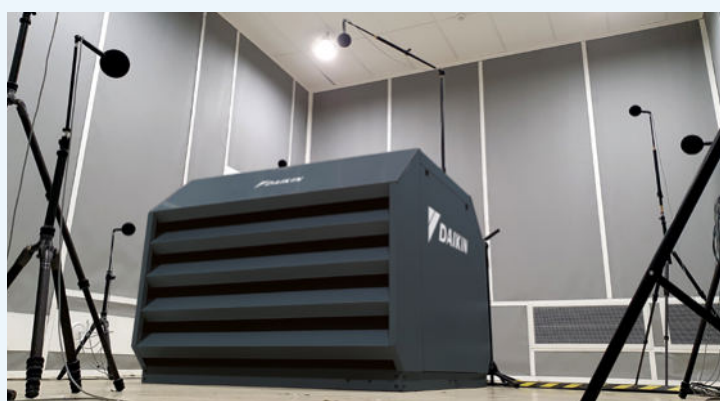
Sound power level measurement in acoustic chamber
