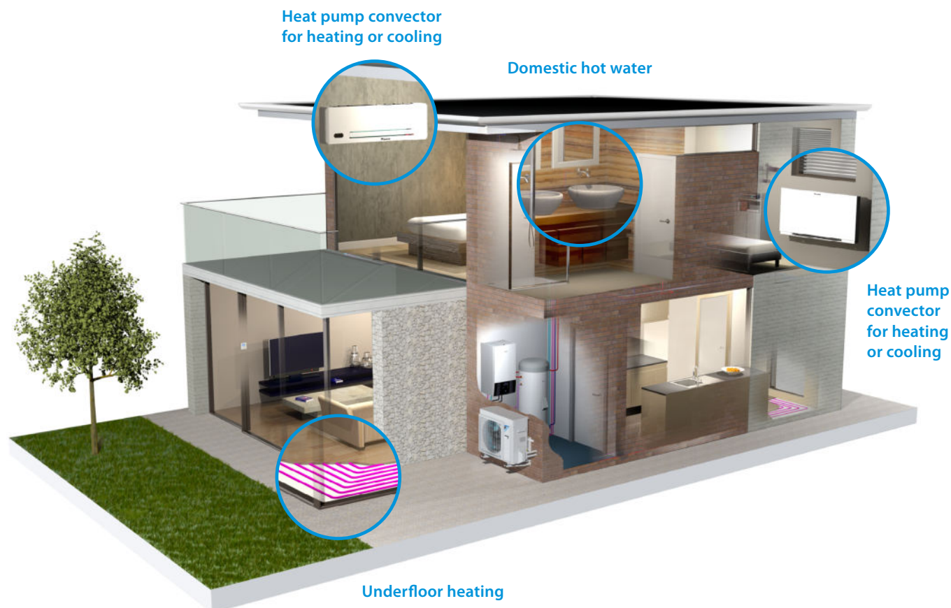
Example of installation with a stainless steel domestic hot water tank (EKHWS(P)-D).
